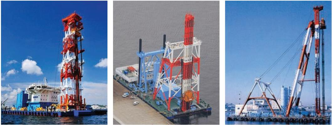
Fig. 16 – Equipamentos do método CDM (*Cement Deep Mixing*) usados em obras *offshore* no Japão (Cement Deep Mixing Method Association, [http://www.cdm-gr.com/sea/ship\\_03.html](http://www.cdm-gr.com/sea/ship_03.html). Acedido em 10/out/2016).
