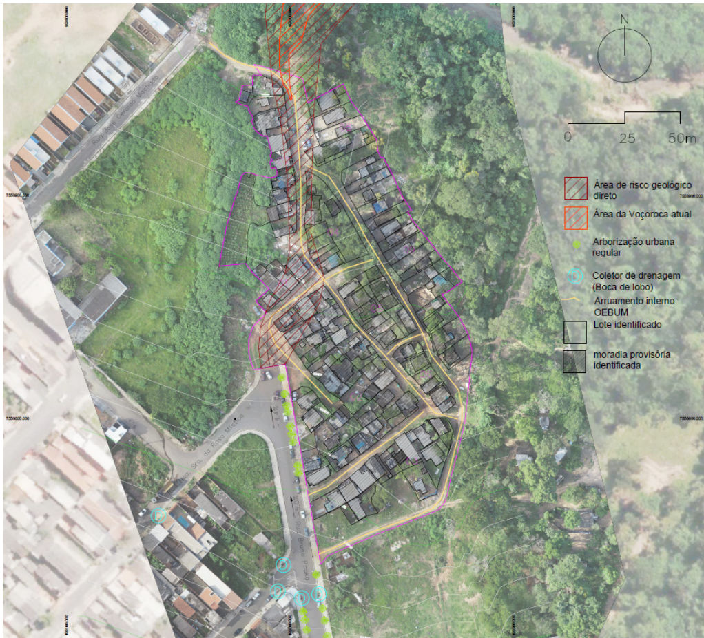
FIGURE 2. Orthophoto taken with an RPA (Remotely Piloted Aircraft) of OEBUM, overlaid on the Google Earth Pro database composed of satellite images, with the gully marked in red.
