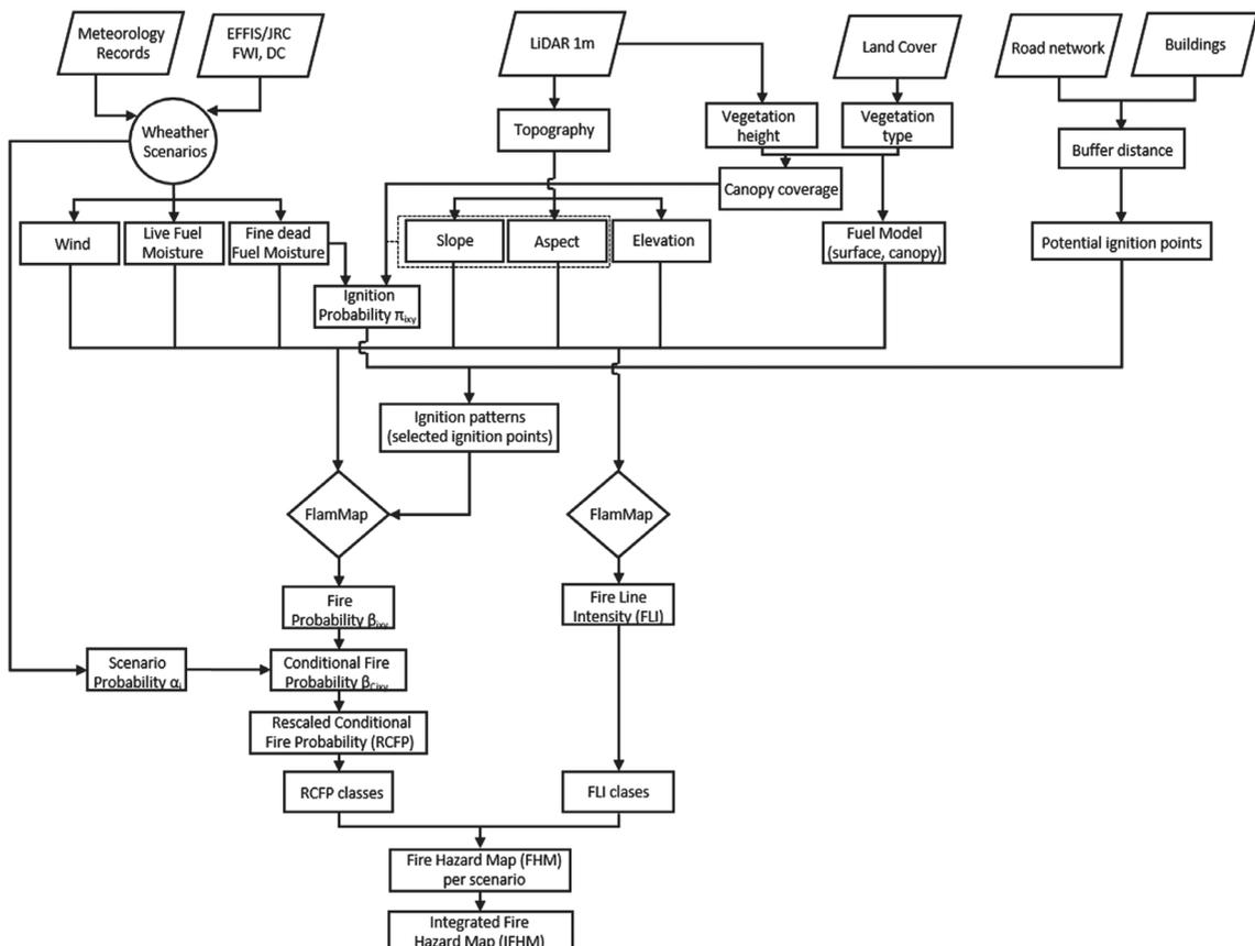
Fig. 4 - Scheme/workflow of the proposed fire hazard model.
